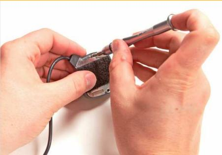
Removing a few Phillips screws allows us to access the innards of the GPS antenna.
