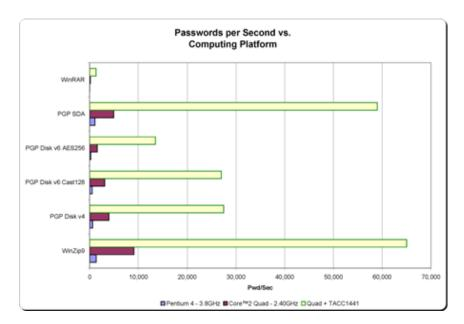
WinRAR, PGP, and WinZip are widely used file formats which present enormous challenges for password recovery software running on traditional processing platforms. As the chart shows, the TACC1441 accelerates each of these algorithms by a factor of 6x - 30x, compared to the un-accelerated processors. For even faster performance than the gain offered by a single TACC1441, use multiple TACC1441 units together on a single computer.
