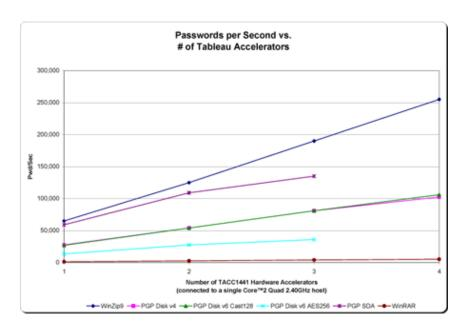
Dictionary-based password attacks, like WinZip, process at rates of 1,000 - 3,000 passwords per second on Pentium IV computers, allowing approximately 20k+ passwords per second on a mid-size DNA cluster. A single CPUs with four TACC1441 accelerators runs in excess of 250,000 passwords per second!
