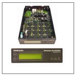
The TACC1441 Hardware Accelerator is the latest innovation. Designed to accelerate the dictionary-based attacks of leading password recovery applications, such as AccessData's Password Recovery Toolkit (PRTK) and Distributed Network Attack (DNA), the TACC1441 increases decryption up to 60 times of non-accelerated systems.
