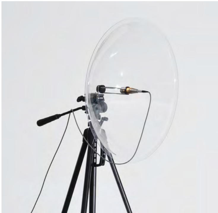
Figure 5: Parabolic microphone: Brüel&Kjær 4145 microphone capsule and 2669 preamplifier, in front of a transparent parabolic reflector (56 cm diameter), using a self-built attachment, on a tripod.
