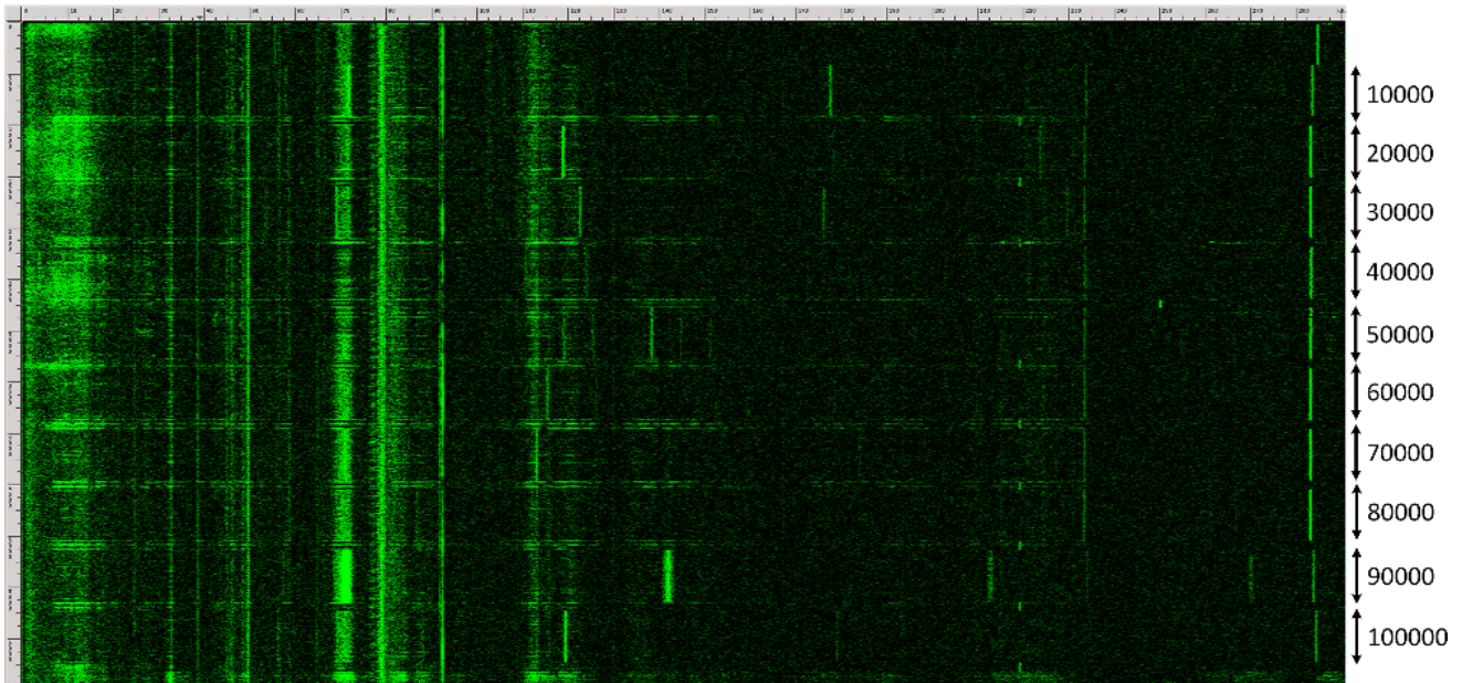
Figure 9: Acoustic signature (6 sec, 0–300 kHz) of loops in different lengths of ADD instructions executed on the Evo N200. The loop length is indicated next to its acoustic signature. The recording was performed using the lab-grade setup and the Brüel&Kjær 4939 high-frequency microphone capsule.
