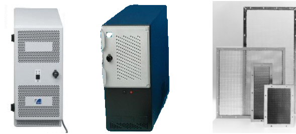
Figure 1: Examples of electromagnetic shielding. The two computers meet the strict NSTISSAM TEMPEST/1-92 Level I requirements for electromagnetic side-channel emanations, yet have ample ventilation holes (catalog photos, left: Advanced Programs, Inc. model DWT-105; middle: EMCON Emission Control Limited Core 2 Quad workstation). On the right are shielded honeycomb air vents (Parker Chomerics CHO-CELL panels of several sizes, “especially designed for high frequency environments and to meet TEMPEST specifications”).
