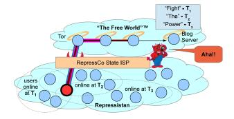
Figure 4: Example of an intersection attack
