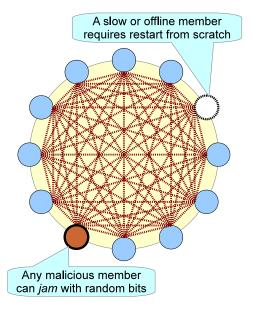
Figure 7: Why DC-nets is hard to scale in practice: (1) worst-case  $N \times N$  coin-sharing matrix; (2) network churn requires rounds to start over; (3) malicious members can anonymously jam the group.
