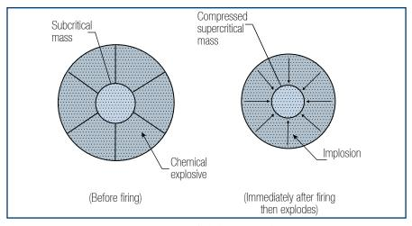
Figure A.9 NAS-2 Unclassified Illustration of an IA Weapon
