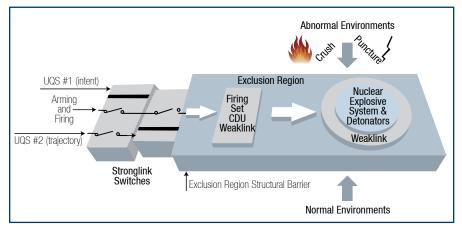
Figure 5.2 Modern Nuclear Safety Architecture
