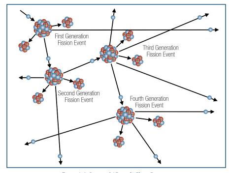
Figure A.5 Sustained (Critical) Chain Reaction
