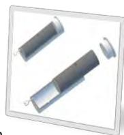
The tamper-evident tube consists of an outer tube with cap, an inner tube with cap, an inner tube locking mechanism, and an outer tube locking mechanism that is affixed to the peripheral surface of the outer cap.
