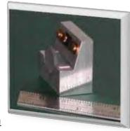
This technology uses an angled sample holder and a two-stage reflector to obtain a perspective view of the sample. A perspective view allows details along the edge to be imaged. Furthermore, the high tilt angle causes as many as 50% of the high energy electrons to be forward scattered off the surface of the sample. These electrons carry high resolution and surface sensitive information.
