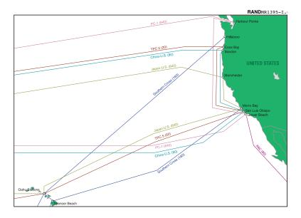
Figure I.6—Submarine Cables Terminating on the West Coast
