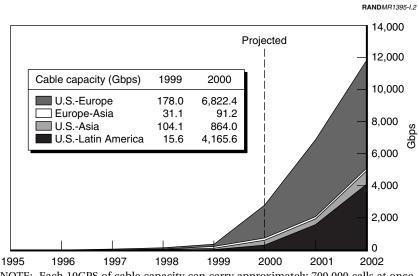
NOTE: Each 10GPS of cable capacity can carry approximately 700,000 calls at once, assuming that five call paths are derived from each standard 64 Kbps circuit.
